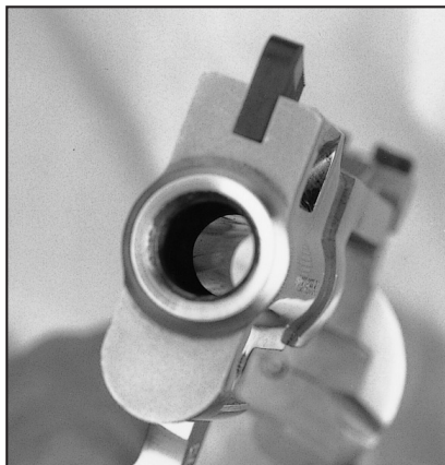
The Rossi's 2.6" barrel sports a full underlug and heavy, solid top rib that houses the revolver's pinned, red insert front sight as well as its eight angled compensator ports.
